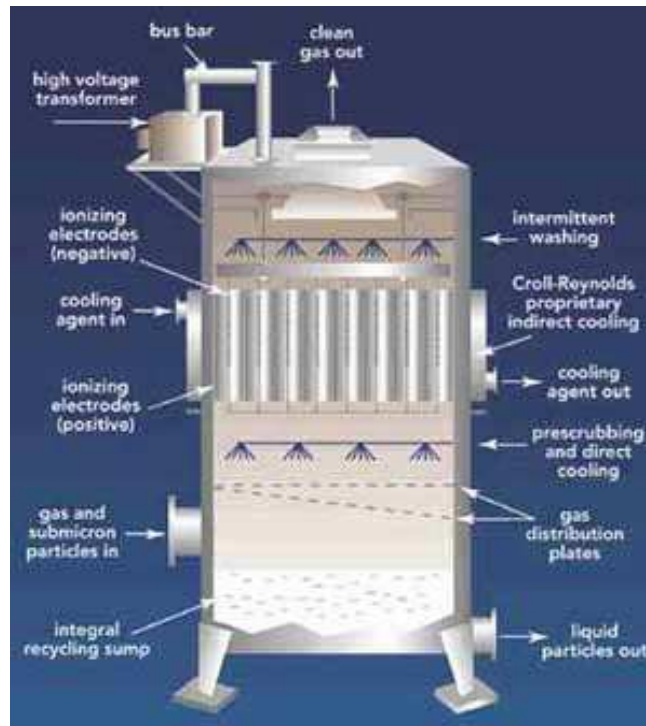
Figure 4-3. Wet ESP [Croll Reynolds]
